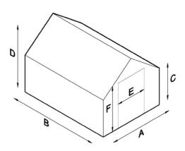
Roof pitch - 36° Snowload - 235 kg/m2 Windload - 41 kg/m2
