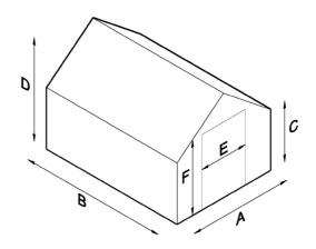
Roof pitch – 36° Snowload – 235 kg/m2 Windload – 41 kg/m2
